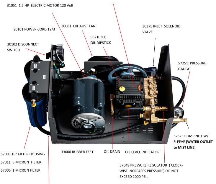
26038 **(WATER INLET)** HOSE 3/8" ID Per ft. 26104 FEMALE GARDEN HOSE ADAPTER. 26042 HOSE SPLICER 3/8" TO EXTEND HOSE
