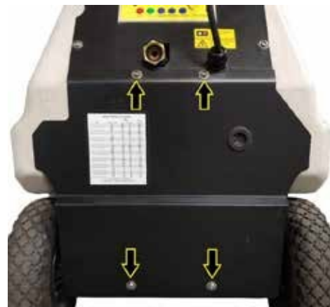
Figure 3 - Back view of the Cool Caddie. The four arrows point to the screws holding the back cover plate onto the unit.
