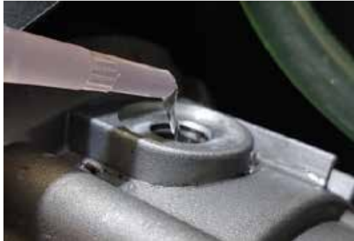
Figure 7 - Horizontal bottle spout filling the pump with oil.
