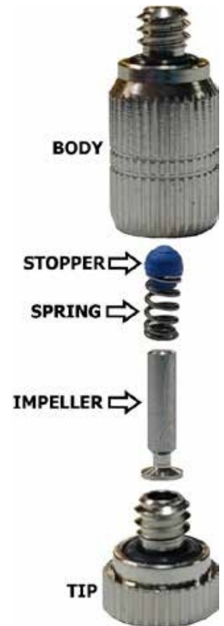
Figure 2 - Exploded view of misting nozzle. Note the anti-drip stopper must not be lost during disassembly.
