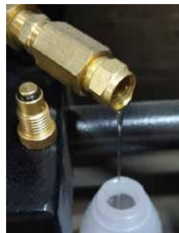
Figure 5 - Oil drain valve with end cap removed.
