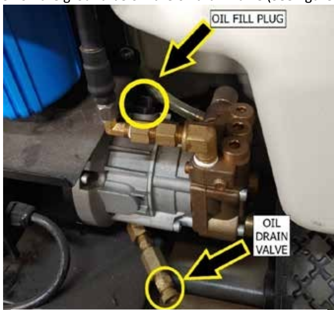
Figure 4 – Oil fill plug and drain valve location.
